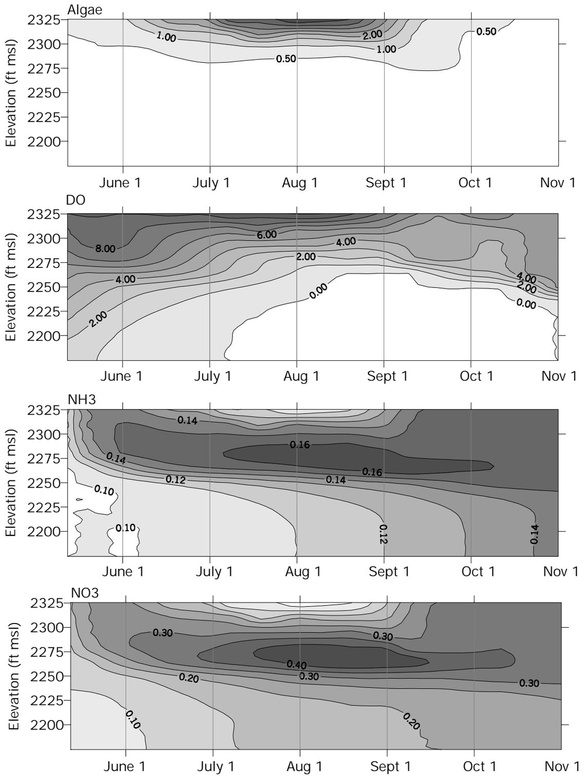
Figure 7.14 Iron Gate Reservoir algae, dissolved oxygen, ammonia (NH<sub>3</sub>), and nitrate (NO<sub>3</sub>) concentrations, June-October 1996. All values in mg/l.
