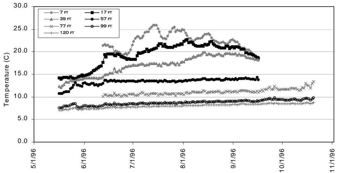
Figure 7.5 Iron Gate Reservoir measured profile water temperature, 1996
