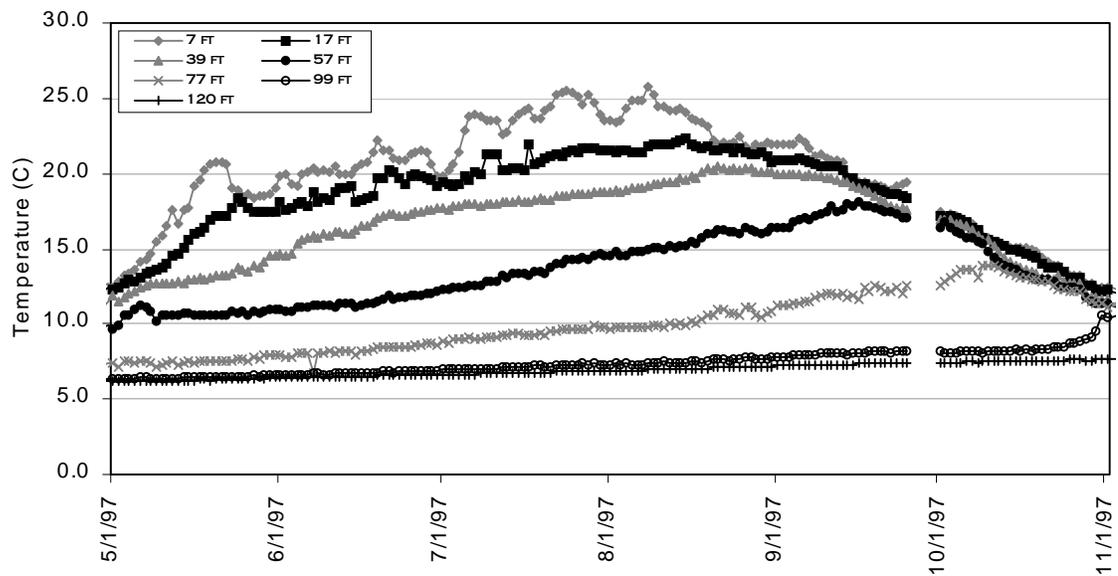
Figure 7.6 Iron Gate Reservoir measured profile water temperature, 1997
