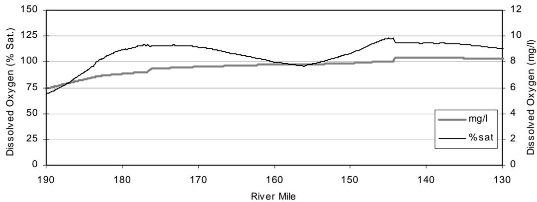
Figure 8.18 Simulated mean daily dissolved oxygen for the Klamath River from Iron Gate Dam to Seiad Valley – baseline: June 15 as percent saturation and mg/l
