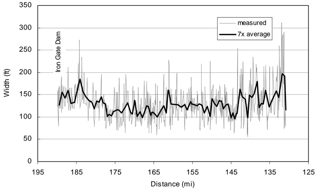
Figure B.1 Measured Klamath River width and 7-times running average, Iron Gate Dam to Seiad Valley
