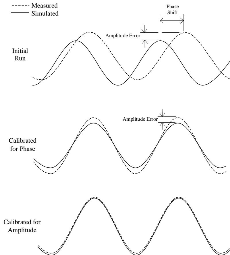
Figure 6.11 Example calibration of phase and amplitude for diurnal temperature trace
